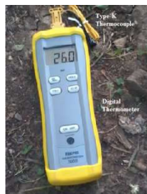
Figure 4: Picture of the Type-K thermocouple (Attached at top) and digital thermometer.
