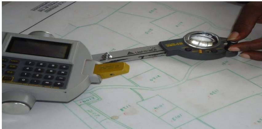
Figure 5: Manual area measurement using a planimeter
