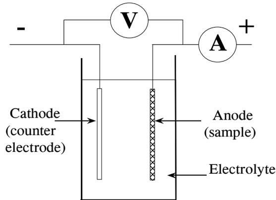
**Figure 1: Schematic diagram for anodization method.**Nemes *et al.*, (2011)
