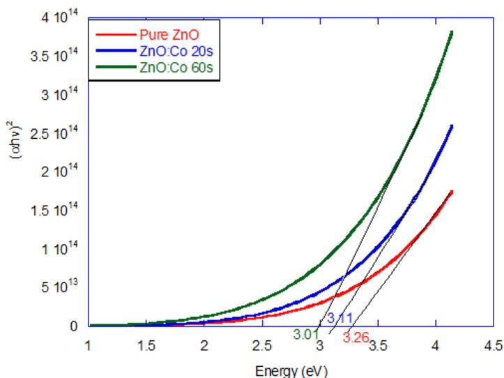
**Figure 6:** Graph showing the optical band gap of the fabricated films
