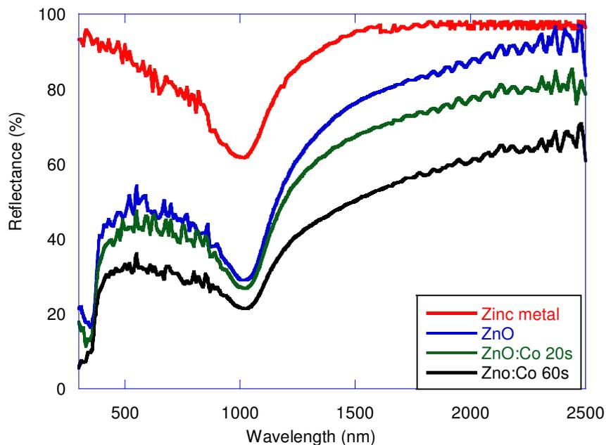
**Figure 4: Measured reflectance spectra for polished zinc metal, pure ZnO and Co:ZnO**
