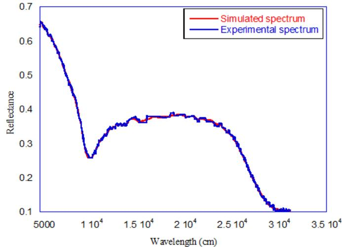
**Figure 2: An illustration of fitting of the experimental to simulated spectra using the SCOUT software**
